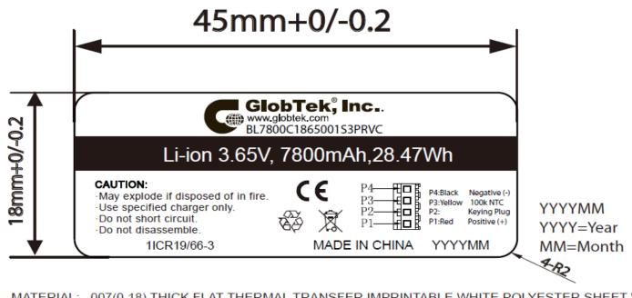
MATERIAL: .007(0.18) THICK FLAT THERMAL TRANSFER, IMPRINTABLE, WHITE POLYESTER SHEET WITH BLACK NOMENCLATURE. LABEL IS GLAZE AND ATTACHED ON PLASTIC CASE. MANUFACTURER: STEVEN LABEL, MATERIAL I.D. NO.3302-33, UL FILE NO.MH12821(N)UL MATERIAL DESIGNATION FILE NO.GHW332RL. OPTIONAL LABEL MATERIAL CAN BE SUBSTITUTED PROVIDING MATERIAL IS UL LISTED AND COMPLIES WITH APPLICABLE SAFETY REQUIREMENTS.
