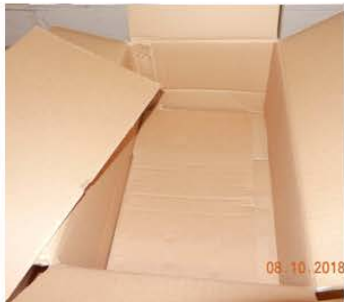
Layer of cardboard added to bottom of master carton
